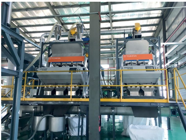
Flake sorters in recycling facility
