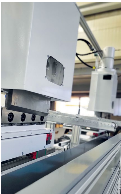
GH systems of the 200 and 300 series from GETECHA during granulation of edge trims below the discharge roller conveyor of an upstream extrusion line
