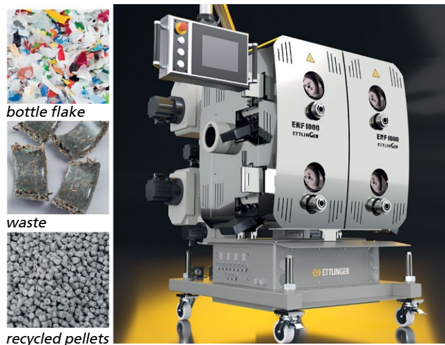
Recycling of PE, PE-HD and PP are among the most common industrial applications of the ERF 1000 continuous melt filter, which can process up to 10 t/h, depending on the material involved (© Ettlenger)
